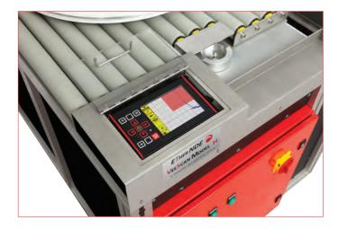
**GREAT EDDY CURRENT TECHNOLOGY:** The VEESCAN works in conjunction with the ETHER NDE AEROCHECK+ eddy current flaw detector. The flaw detector sits behind a protective tough polycarbonate window and provides the unit with the eddy current technology for the inspection.
